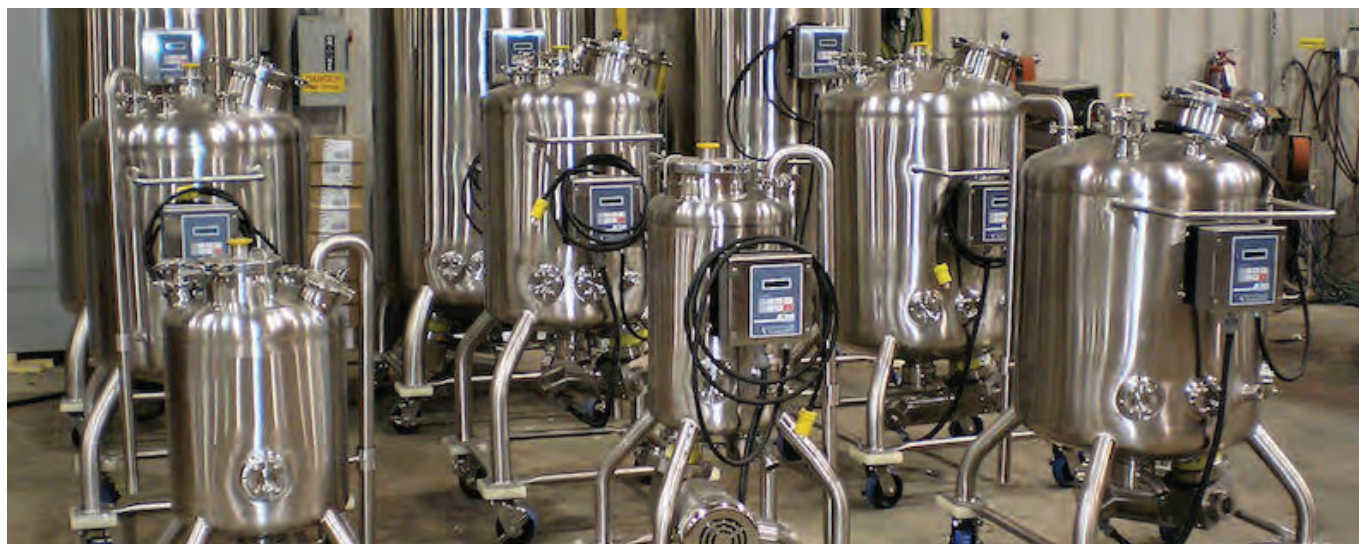
Stainless Fabrication electropolished pharma vessels (50 to 700 litres)
